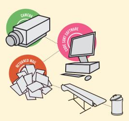
When mail is returned to the sender due to 'Gone Away' or 'Undeliverable' reasons, the return mail system will read the barcode printed on the envelope or within the window of the envelope and create a simple database of records.
